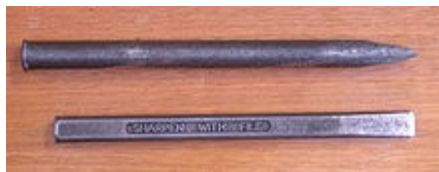
Figure 2.13 Top: Bull point chisel; Bottom: Cold chisel
