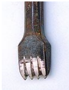
Figure 2.14 A toothed stone chisel
