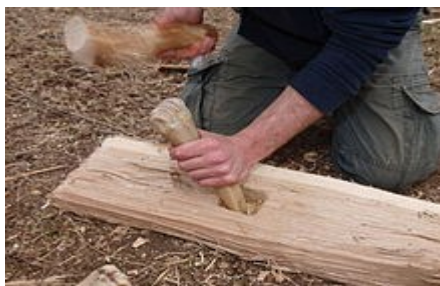
Figure 2.10 Reconstruction chisel made from a robust cow's cannon bone, cutting a mortise
