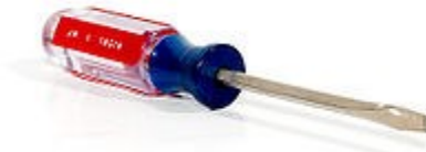
Figure 2.1 A slotted or "flat-blade" screwdriver
