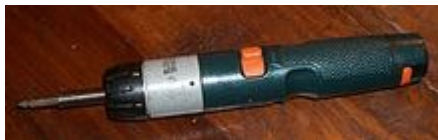
Figure 2.6 A rechargeable battery-powered electric screwdriver
